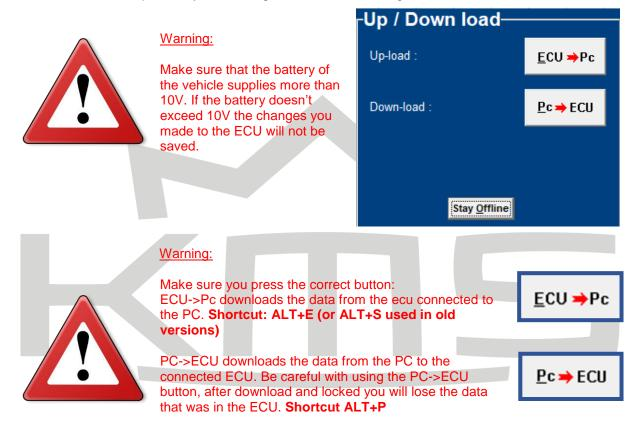
Tip: On vehicles with an ignition lock switched in such a way that the power supply to the system is cut off when the engine is started, always download the data from the PC to the system (as in the PC the modified data will not get lost when the power supply to the system is broken). This is of course only necessary if the data has not been saved to the system.
