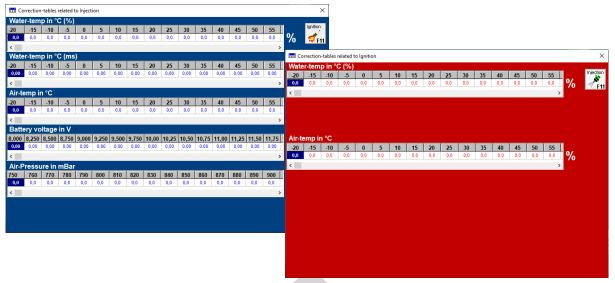
Function key F11 switches between injection correction charts and ignition correction charts.
