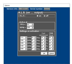
If using variable A.L.S. by connecting a potentiometer signal you can vary the PWM value from 0 to the value set here in the A.L.S. settings. The potentiometer must be in the range of  $1 k\Omega - 47 k\Omega$ . The variable signal from the potentiometer must be connected analog aux input on pin 4. The 5V for the potentiometer can be branched from the 5V sensor supply on pin 14. The remaining pin of the potentiometer must be connected to the ground on pin 17.
