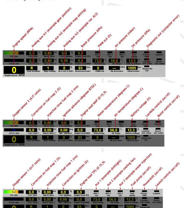
These readings can be used to check whether the right sensors are being used and all settings are correct.
