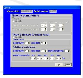
opening speed is needed for initial burst enrichment to occur. The amplifier is more or less a factor for the amount of fuel injected. A higher amplifier results in more enrichment.
