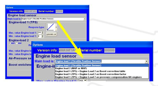
Two engine load sensors called "Engine load 1" (for TPS = throttle position sensor) and "Engine load 2" (for MAP = manifold absolute pressure sensor) can be connected. Even a MAF sensor (mass air flow meter) can be connected (not recommended). Please note that certain combinations will result in the exclusion of some options.
