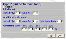
opening speed of the throttle. A low value for sensitivity means that the initial burst won't occur fast, a high throttle opening speed is needed. For a high sensitivity value a lower throttle
