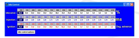
This function (idle-control) will show tables and parameters, where you can adjust the fuelling in ms, ignition in degree advance and opening of the idle-valve in %. (500 - 1250rpm)
