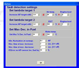
EGT  $\rightarrow$  CAN converter is connected, input 1 will be the EGT used for the fuel correction. Recommended: -0.5 - -1.5.
