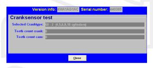
If another reading is shown, check whether the sensor is correctly connected and properly mounted. Electronic interference can occur when the leads are not properly shielded or positioned close to the coil and spark leads. A sensor taking a reading from an external cog may have metal particles attached to it as a result of grinding or drilling. If a failure only starts occurring at higher engine speeds, it is likely that it is caused by sensor vibrations.
