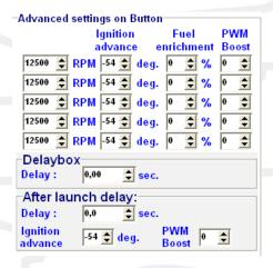
The 'Delay Box' is a special timing parameter for the launch control. The timer is activated when the launch control button is released. During the countdown of the timer, the launch control settings are still active meaning that the engine will continue the launch control limit for the entire duration of the timer. Setting the delay to 0 seconds means that the launch control limit is ended at the exact moment that the launch control button is released.
