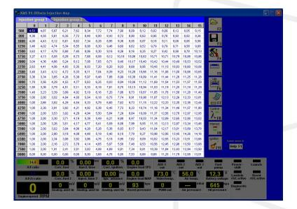
You can switch between injector groups (when activated, see section 3.2.4.1.4 Injection settings) by clicking on the buttons that are marked in the drawing below. These groups can be set for different kind of injector banks. For more settings look at the hardware configuration and the injection settings (see 3.2.4.1.7 Hardware configuration and 3.2.4.1.4 Injection settings).
