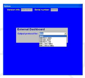
Specially for AIM dashboards, there are communication protocols in the KMS software. Users can choose between AIM PROT\_UART, AIM KMS\_UART and AIM PROT\_CAN. Select in the AIM Racestudio2 software the configuration with the correct ECU manufacturer (AIM or KMS) and model (PROT\_UART, KMS\_UART or PROT\_CAN).
