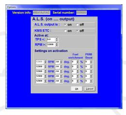
If using variable A.L.S. by connecting a potentiometer signal you can vary the PWM value from 0 to the value set here in the A.L.S. settings. The potentiometer must be in the range of 1 k $\Omega$  - 47 k $\Omega$ . The variable signal from the potentiometer must be connected analog aux2 input on pin 25 or analog aux3 input on pin 24. The 5V for the potentiometer can be branched from the 5V sensor supply on pin 20. The remaining pin of the potentiometer must be connected to the ground on pin 23.
